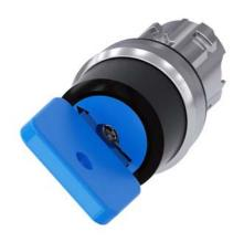
Key-operated switch O.M.R, 22 mm, round, metal, shiny, lock number 73038, blue, with 2 keys, 2 switch positions O-I, latching, actuating angle 90°, 10:30h/13:30h, key removal O, with laser labeling, upper case and lower case, always upper case at beginning of line
