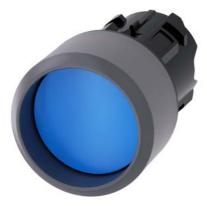
Pushbutton, 22 mm, round, plastic with metal front ring, blue, Front ring, raised momentary contact type, with laser labeling, symbol number according to, ISO 7000 or IEC 60417
