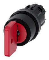
Key-operated switch O.M.R, 22 mm, round, plastic, lock number 73037, red, with 2 keys, 3 switch positions I-O-II, latching, actuating angle 2x45°, 10:30h/12h/13:30h, key removal O+I, with laser labeling, upper case
