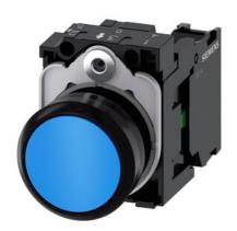
Pushbutton, 22 mm, round, plastic, blue, pushbutton, flat, momentary contact type, with holder 1 NO, screw terminal, with laser labeling, upper case and lower case, always upper case at the beginning of the word
