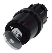
Key-operated switch BKS, 22 mm, round, plastic, lock No. E9 (VW), without key, 2 switch positions O-I, latching, actuating angle  $90^\circ$ , 10:30h/13:30h, key removal O+I, with laser labeling, lower case
