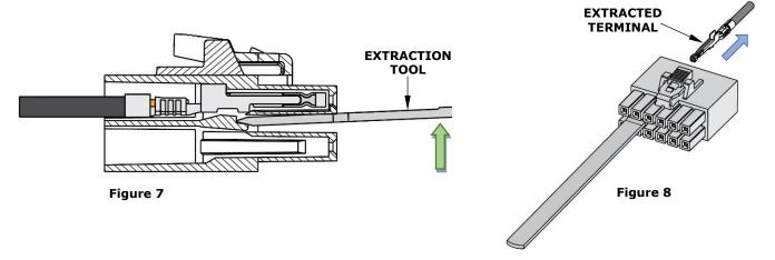
6. Pull the terminated wire out of the connector housing in the direction of the arrow. See Figure 8.
