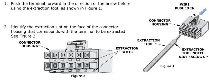
3. Hold the extraction tool so that the notched side faces up. Insert the extraction tool into the correct extraction slot, keeping the tip of the extraction tool pointing up and against the top of the extraction slot. See Figures 3 and 4.
