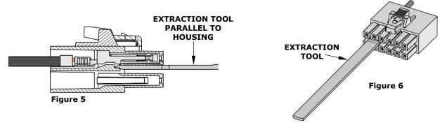
5. While holding the housing and wire in place, lift up on the extraction tool handle so that the tip of the tool pushes downward on the extraction slot. See Figure 7. This will allow the terminal to move freely inside the connector slot.
