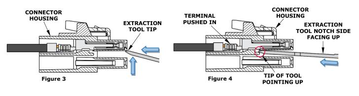
Ultra-Fit Tangless Crimp Terminal Extraction Tool
