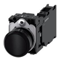
Pushbutton, 22 mm, round, plastic, black, pushbutton, flat, momentary contact type, with holder 1 NO+1 NC, spring-type terminal, with laser labeling, upper case and lower case, always upper case at the beginning of the word
