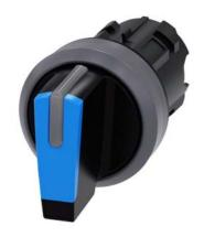
Selector switch, illuminable, 22 mm, round, plastic with metal front ring, blue, selector switch, short, 3 switch positions I>O<II, momentary contact type, actuating angle  $2x45^{\circ}$ , 10:30h/12h/13:30h, with laser labeling, upper case and lower case, always upper case at the beginning of the word
