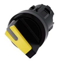
Selector switch, illuminable, 22 mm, round, plastic, yellow, selector switch, short, 2 switch positions O-I, latching, actuating angle  $90^\circ$ , 10:30h/13:30h, with laser labeling, upper case
