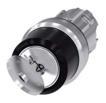
RONIS key-operated switch, 22 mm, round, metal, shiny, lock number SB30, with 2 keys, 2 switch positions O<I, momentary contact type, Actuating angle  $45^\circ$ , 10:30h/12h, key removal O, possible special locks: SB31, 421, 455, with laser labeling, upper case
