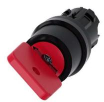
Key-operated switch O.M.R, 22 mm, round, plastic, lock number 73037, red, with 2 keys, 2 switch positions O<I, momentary contact type, Actuating angle 45°, 10:30h/12h, key removal O, with laser labeling, upper case and lower case, always upper case at the beginning of the word
