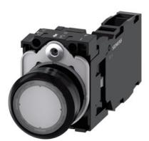
Pushbutton, 22 mm, round, plastic, clear, pushbutton, flat, momentary contact type, with holder 1 NO+1 NC, screw terminal, with laser labeling, upper case and lower case, always upper case at beginning of line
