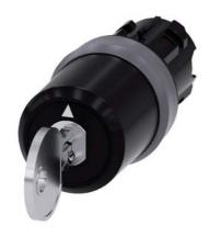
key-operated switch Siemens, 22 mm, round, plastic with metal front ring, lock number SSG10, with 2 keys, 3 switch positions I-O-II, latching, actuating angle  $2x45^{\circ}$ , 10:30h/12h/13:30h, key removal II, with laser labeling, upper case and lower case, always upper case at the beginning of the word
