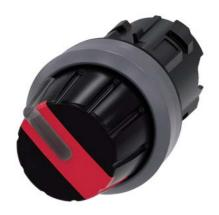
Selector switch, illuminable, 22 mm, round, plastic with metal front ring, red, Rotary knob, 2 switch positions O-I, latching, actuating angle 90°, 10:30h/13:30h, Z=50-unit packaging
