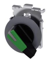
Selector switch, illuminable, 30 mm, round, Metal, matte, green, selector switch, long, front ring for flush installation, 2 switch positions O<I, momentary contact type, Actuating angle 45°, 10:30h/12h, with laser labeling, upper case and lower case, always upper case at the beginning of the word
