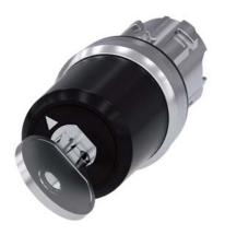
Key-operated switch BKS, 22 mm, round, metal, shiny, lock number S1, with 2 keys, 2 switch positions O-I, latching, actuating angle  $90^\circ, 10:30h/13:30h,$  key removal O, with laser labeling, upper case and lower case, always upper case at the beginning of the word
