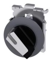
Selector switch, illuminable, 30 mm, round, Metal, matte, white, selector switch, short, front ring for flush installation, 2 switch positions O-I, latching, actuating angle  $90^{\circ}$ , 10:30h/13:30h, with laser labeling, lower case
