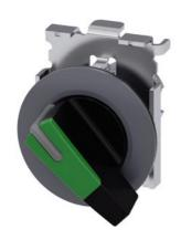
Selector switch, illuminable, 30 mm, round, Metal, matte, green, selector switch, long, front ring for flush installation, 2 switch positions O-I, latching, actuating angle  $90^\circ,\,10:\!30h/13:\!30h,$  with laser labeling, upper case and lower case, always upper case at the beginning of the word
