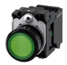
Illuminated pushbutton, 22 mm, round, plastic, green, pushbutton, flat, momentary contact type, with holder, 1NO, LED module with integrated LED 24 V AC/DC, spring-type terminal, with laser labeling, lower case
