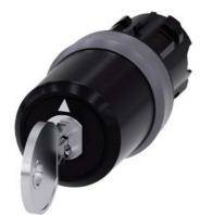
key-operated switch Siemens, 22 mm, round, plastic with metal front ring, lock number SSG10, with 2 keys, 3 switch positions I-O-II, latching, actuating angle  $2x45^{\circ}$ , 10:30h/12h/13:30h, key removal I+O+II, with laser labeling, upper case and lower case, always upper case at beginning of line
