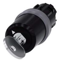
key-operated switch Siemens, 22 mm, round, plastic with metal front ring, lock number SSG10, with 2 keys, 2 switch positions O<I, momentary contact type, actuating angle 45°, 10:30h/12h, key removal O, Z=50-unit packaging
