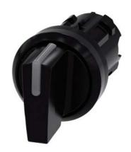
Illuminable selector switch, 22 mm, round, plastic, black, Selector switch short, 3 switch positions I>O<II, momentary contact on the left, latching on the right, actuating angle 2x45°, 10:30 /12 /13:30, Z=50-unit packaging
