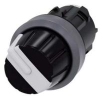
Selector switch, 22 mm, round, plastic with metal front ring, white, Rotary knob, 4 switch positions I-II-III-IV, latching, Actuating angle  $4x90^\circ, 3h/6h/9h/12h,$  with laser labeling, upper case
