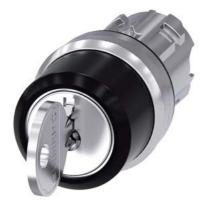
RONIS key-operated switch, 22 mm, round, metal, shiny, lock number SB30, with 2 keys, 3 switch positions I-O<II, left latching, right momentary contact type, actuating angle 2x45°, 10:30h/12h/13:30h, key removal O+I, possible special locks: SB31, 421, 455, with laser labeling, upper case and lower case, always upper case at beginning of line
