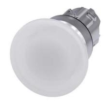
Illuminated mushroom pushbutton, 22 mm, round, metal, shiny, white, 40 mm, momentary contact type, with laser labeling, symbol number according to, ISO 7000 or IEC 60417
