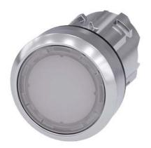
Illuminated pushbutton, 22 mm, round, metal, shiny, white, pushbutton, flat, latching, Push-to-release mechanism, with laser labeling, symbol number according to, ISO 7000 or IEC 60417
