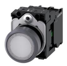
Illuminated pushbutton, 22 mm, round, plastic with metal front ring, white, pushbutton, flat, momentary contact type, with holder, 1NO, LED module with integrated LED 230 V AC, screw terminal, with laser labeling, upper case
