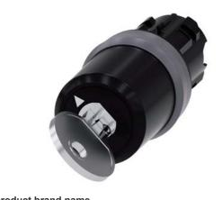
key-operated switch Siemens, 22 mm, round, plastic with metal front ring, lock no. LSG1, with 2 keys, 2 switch positions O-I, latching, actuating angle 90°, 10:30h/13:30h, key removal O, with laser labeling, upper case and lower case, always upper case at beginning of line
