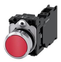
Pushbutton, 22 mm, round, metal, shiny, red, pushbutton, flat, momentary contact type, with holder, 1 NO+1 NC, spring-type terminal, with laser labeling, upper case and lower case, always upper case at the beginning of the word
