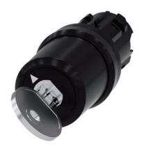
Key-operated switch BKS, 22 mm, round, plastic, Lock No. E7 (VW), without key, 2 switch positions O-I, latching, actuating angle  $90^\circ, 10:30h/13:30h,$  key removal O, with laser labeling, upper case and lower case, always upper case at the beginning of the word
