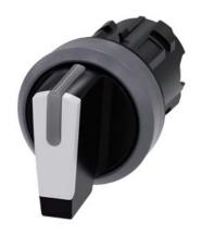
Selector switch, illuminable, 22 mm, round, plastic with metal front ring, white, selector switch, short, 3 switch positions I>O<II, momentary contact on the left, latching on the right, actuating angle 2x45°, 10:30h/12h/13:30h, with laser labeling, inscription or symbol Customer-specific selection with SIRIUS ACT configurator (CIN)
