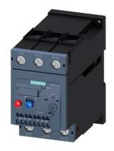
Overload relay 36...45 A Thermal For motor protection Size S2, Class 10 Stand-alone installation Main circuit: Screw Auxiliary circuit: spring-type terminal Manual-Automatic-Reset
