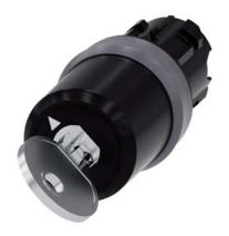
key-operated switch Siemens, 22 mm, round, plastic with metal front ring, special lock, with 2 keys, 2 switch positions O-I, latching, actuating angle  $90^\circ,\,10:\!30h/13:\!30h,$  key removal O
