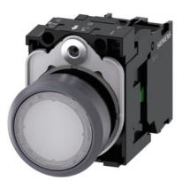
Illuminated pushbutton, 22 mm, round, plastic with metal front ring, white, pushbutton, flat, momentary contact type, with holder, 1NO, LED module with integrated LED 230 V AC, screw terminal, with laser labeling, upper case and lower case, Always upper case at the beginning of the word
