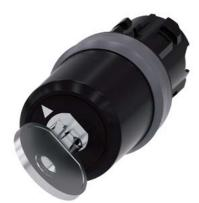
Key-operated switch BKS, 22 mm, round, plastic with metal front ring, lock No. E9 (VW), without key, 2 switch positions O-I, latching, actuating angle  $90^{\circ}$ , 10:30h/13:30h, key removal O+I, with laser labeling, lower case
