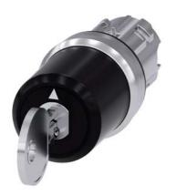
key-operated switch Siemens, 22 mm, round, metal, shiny, lock no. STGH10, with 2 keys, 3 switch positions I-O<II, left latching, momentary contact type on the right, actuating angle 2x45°, 10:30h/12h/13:30h, key removal O+I, with laser labeling, inscription or symbol customer-specific selection with SIRIUS ACT configurator (CIN)
