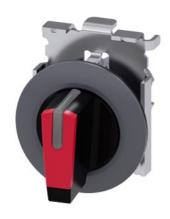
Selector switch, illuminable, 30 mm, round, Metal, matte, red, selector switch, short, front ring for flush installation, 3 switch positions I>O<II, momentary contact type, actuating angle 2x45°, 10:30h/12h/13:30h, with laser labeling, upper case and lower case, always upper case at beginning of line
