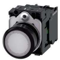
Illuminated pushbutton, 22 mm, round, plastic, white, pushbutton, flat, momentary contact type, with holder, 1NO, LED module with integrated LED 110 V AC, screw terminal, with laser labeling, upper case
