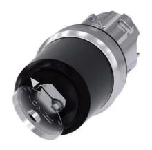
Key-operated switch IKON, 22 mm, round, metal, shiny, lock number 360012K1, with 2 keys, 2 switch positions O<I, momentary contact type, Actuating angle 45°, 10:30h/12h, key removal O, with laser labeling, upper case and lower case, always upper case at beginning of line
