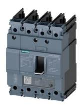
circuit breaker 3VA5 UL frame 125 breaking capacity class H 65kA @ 480V 4-pole, line protection TM230, FTAM, In=40A overload protection Ir=40A fixed short-circuit protection Ii=5...10 x In N conductor unprotected without connection
