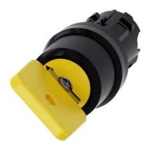
Key-operated switch O.M.R, 22 mm, round, plastic, lock number 73033, yellow, with 2 keys, 2 switch positions O-I, latching, actuating angle 90°, 10:30h/13:30h, key removal O+I, with laser labeling, upper case and lower case, always upper case at beginning of line
