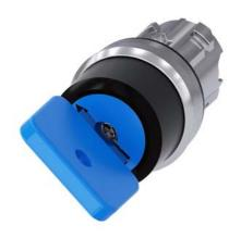
Key-operated switch O.M.R, 22 mm, round, metal, shiny, lock number 73038, blue, with 2 keys, 2 switch positions O<I, momentary contact type, Actuating angle 45°, 10:30h/12h, key removal O, with laser labeling, lower case
