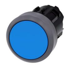
Pushbutton, 22 mm, round, plastic with metal front ring, blue, pushbutton, flat, latching, Push-to-release mechanism, with laser labeling, lower case
