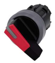
Selector switch, illuminable, 22 mm, round, plastic with metal front ring, red, selector switch, long, 2 switch positions O-I, latching, actuating angle  $90^\circ,\,10:30h/13:30h,$  with laser labeling, lower case
