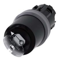
Key-operated switch IKON, 22 mm, round, plastic with metal front ring, lock number 360012K1, with 2 keys, 2 switch positions O-I, latching, actuating angle  $90^{\circ}$ , 10:30h/13:30h, key removal O, with laser labeling, lower case
