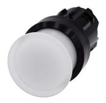
Illuminated mushroom pushbutton, 22 mm, round, plastic, white, 30 mm, momentary contact type, with laser labeling, upper case and lower case, always upper case at the beginning of the word
