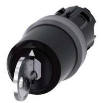
Key-operated switch IKON, 22 mm, round, plastic with metal front ring, lock number 360012K1, with 2 keys, 3 switch positions I>O<II, momentary contact type, actuating angle 2x45°, 10:30h/12h/13:30h, key removal O, with laser labeling, upper case
