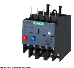
Overload relay 0.22...0.32 A Thermal For motor protection Size S00, Class 10 Contactor mounting Main circuit: Ring cable lug Auxiliary circuit: ring cable lug Manual-Automatic-Reset
