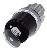
Key-operated switch BKS, 22 mm, round, metal, shiny, lock number S1, with 2 keys, 2 switch positions O<I, momentary contact type, Actuating angle 45°, 10:30h/12h, key removal O, with laser labeling, lower case
