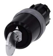
Key-operated switch BKS, 22 mm, round, plastic with metal front ring, special lock, with 2 keys, 3 switch positions I>O<II, momentary contact on the left, latching on the right, actuating angle 2x45°, 10:30h/12h/13:30h, key removal O, Note: BKS locking systems E1 ... E27 supplied without key
